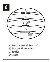
Locate the factory wiring harness in the dash. Metra recommends making connections as shown using the supplied wire harness. (Isolate and individually tape off the ends of any unused wires to prevent electrical short circuit).
